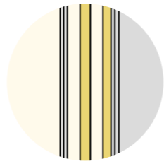
4. Additional layer of acoustic insulation and plasterboard
