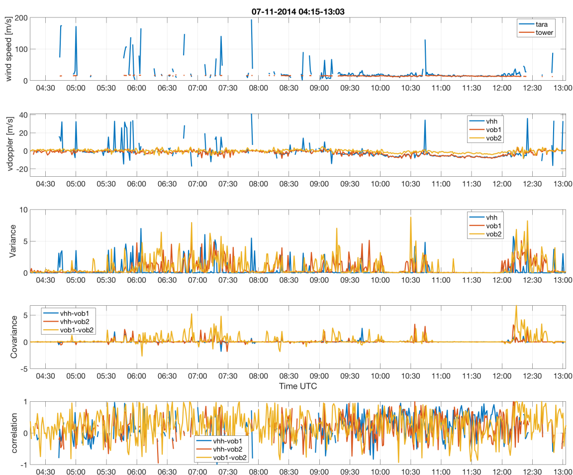
Figure 4.18: This figure includes five plots of the same time series on the 7.11.2014. The top plot shows the wind speed estimate of TARA as well as the measurement of the tower. The second plot shows the 1-minute averaged mean Doppler velocities. The plot in the middle shows the variances over 1 minute for the mean Doppler velocities of the three beams. The fourth plot shows the covariance of the three beams. The last plot shows the correlations for the mean Doppler velocities between the three beams.
