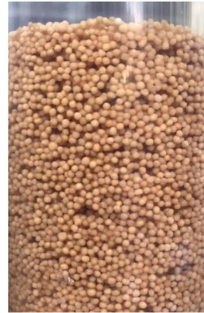
Fig. 3. Fluidised calcite pellets in water at normal fluidisation: voids are clearly visible (1.4–1.7 mm 20 °C, 0.022 m/s).
