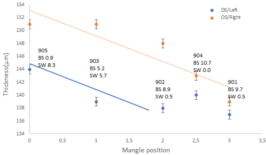
Figure 1.14: The relationship between the mangle gap and the thickness of the glue with indications about the number of sand wrinkle defects per meter
