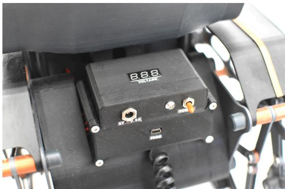
Figure D.5: The switch box and control box of the OctoWalker.
