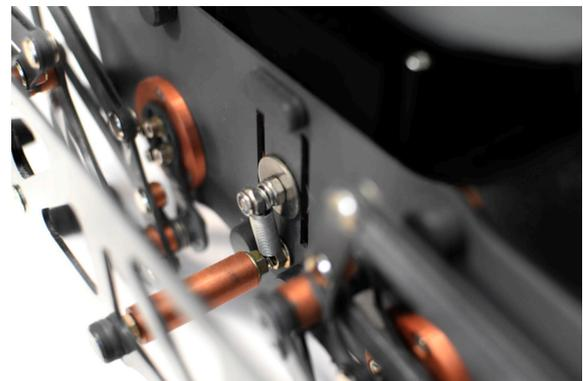
Figure D.6: The belt tensioner of the OctoWalker.
