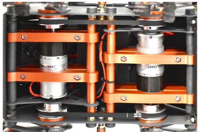
**Figure 5.6:** Bottom inside view of the chassis, in which two DC motors are connected to two lead gears; and two follower gears are connected to the follower gear frame. Each lead gear was connected to a follower gear by a timing belt, which is tensioned by a belt tensioner. Tie wraps were used for cable management, such that the cables do not touch the rotating components of the DC motors and gears.
