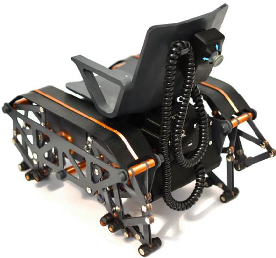
**Figure 5.8:** Back isometric view of the OctoWalker, in which the chair, safety shields, electronic boxes, joystick and mudguards were placed.
