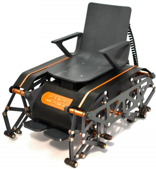
**Figure 5.7:** Front isometric view of the complete OctoWalker, in which the chair, safety shields and mudguards were placed.
