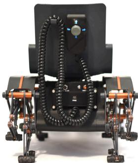
Figure D.3: Back view of the OctoWalker with joystick attached to chair using velcro.
