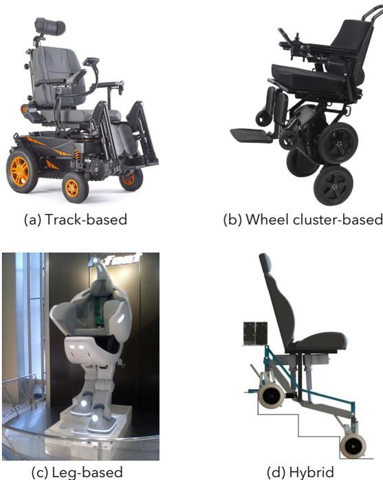
**Figure 1.2:** Examples of stair-climbing electric powered wheelchairs (EPWs) include (a) the track-based EPW of TopChair-S [14]; (b) the wheel cluster-based EPW of iBOT [15]; (c) the leg-based EPW of Toyota I-foot [16]; and (d) the hybrid EPW of Chocoteco et al. (2015) [17].
