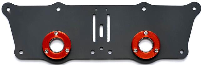
**Figure 5.4:** Before assembling the legs to the two inner and outer frames, the bearing houses were assembled to the inner frames. The outer houses and bearings of the bearing houses were attached to the inner frames with three M3 flat-headed bolts and nuts.
