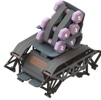
**Figure 6.12:** Dumbbell stacking for the payload test (T4) with each dumbbell weighing 1 kg. The numbers indicate the order, in which the dumbbells were stacked and fixed to the chair.
