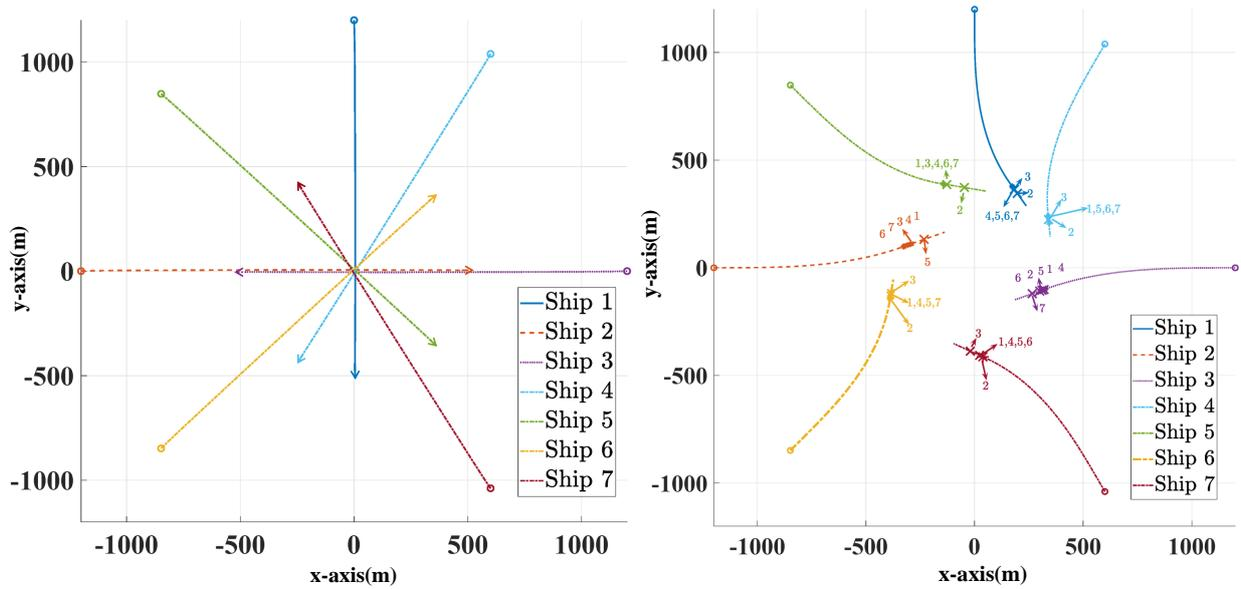
Figure 6: Simulated trajectories of 7 ships with original courses.
