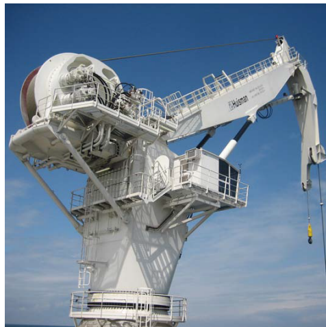
Figure 1.2: 120 meter hydraulic crane, built by Huisman and controlled by the HMC
