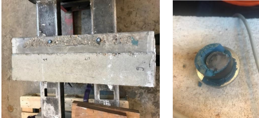
Figure 3.21: Specimen failed due to shear failure of the bolts
