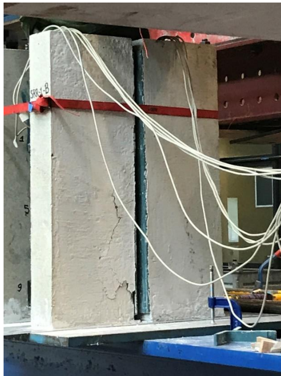
Figure 3.17: Concrete cracks during test SRR1
