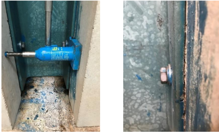
Figure 3.19: Creation of gap in steel-concrete interface
