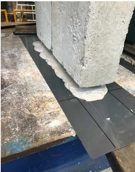
c) Placement of the PVCs under the specimen
