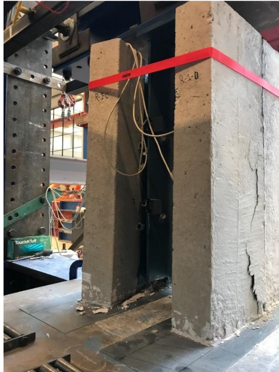
Figure 3.13: Concrete cracks during test R1
