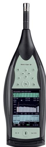
Figure 4.1: Brüel & Kjær hand-held 2250 Sound Level Meter. <sup>1</sup>
