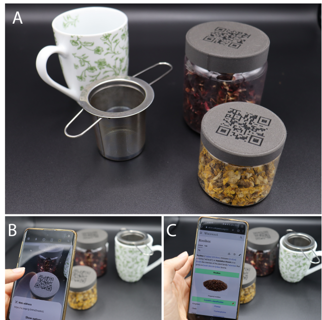
Figure 6: Sufficient color contrast to fabricate readable QR codes A) 3D printed lids with QR codes. B) Scanning the QR code with a mobile phone. C) QR code leads to a webpage sharing information about the herb.
