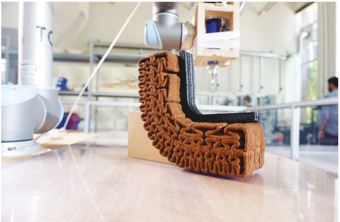
Figure 10: Final 3D-printed window frame.
