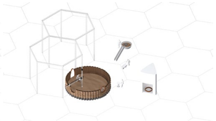
Figure 15: Construction process, printing wooden window frame and 3DP wall simultaneously.
