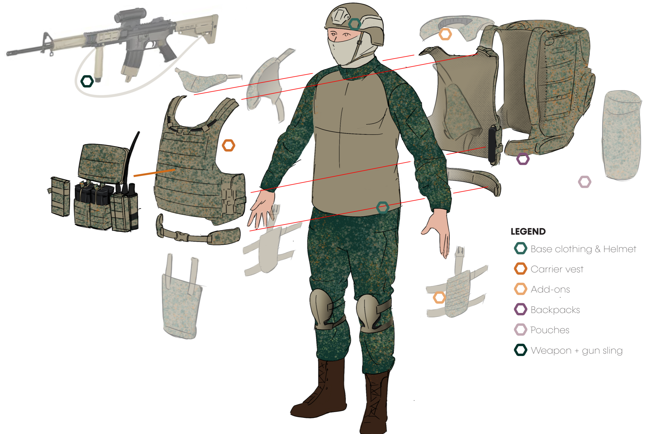
Fig. 10: Exploded view of the various types of legacy equipment on a soldier
