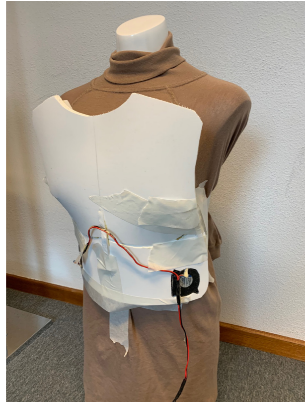
Fig. 52: Airflow distribution test setup Conventional prototype fixation on mannequin
