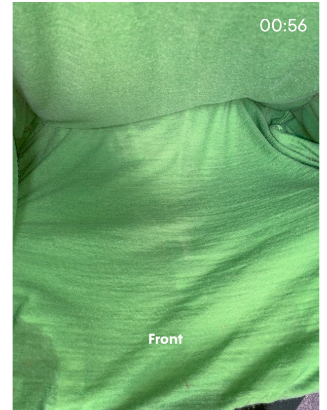
Fig. 66: Humidity check at 56 along the circumference of the vest under the shell. Outside of the area covered by the front shell, the fabric was noticeably more humid, as expected.
