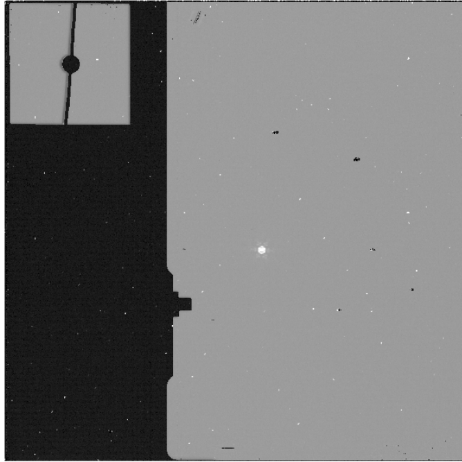
Figure 6.2: Asteroid (2008 UN310), the white circle, is shown in the FOV of the MIRI's imager on the 16.02.2020 at 00:00:00 UTC. The apparent motion of the asteroid is 0.0054 arc/s. The estimated temperature of this asteroid is 204.7 K, the albedo is 0.06 and the exposure time is 49.95 seconds. The black part (structure) of the image is the coronagraphy, as can be seen in Figure 4.4.
