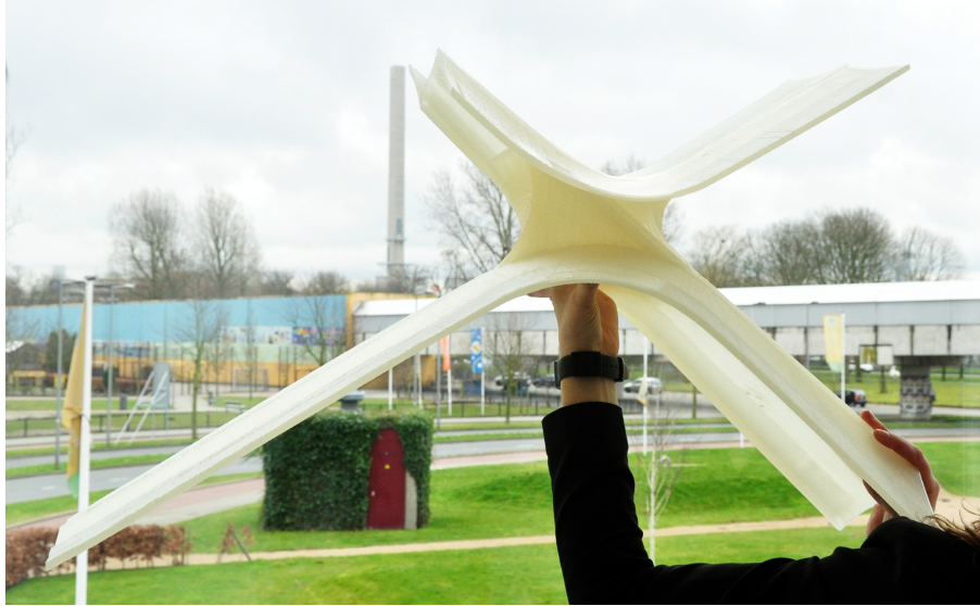
FIGURE 3.8 Physical prototype of a single shading element. Image and design by Ector Hoogstad Architecten & TU Delft/Chair Design Informatics.
