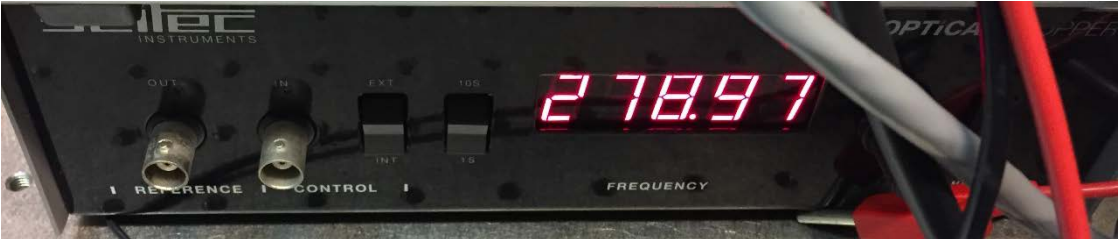
Figure 6.6 Chopping frequency controller
