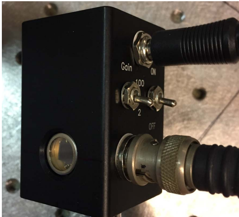
Figure 6.4 Detector with gain options of 2 and 100
