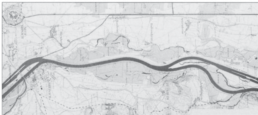
Figure 17 Topographical maps of Upper Rhine channelling (exemplary sections): 1828 - wild river with side arms, branches and gravel banks; 1872 - average width 200 m, doubling average discharge capacity, alluvial forest still flooded; 1963 - Rhine side channel, barrages, dikes directly aligning river bed, disconnection of alluvial forest. (Ministry of Environment Baden-Wuerttemberg, 2007).
