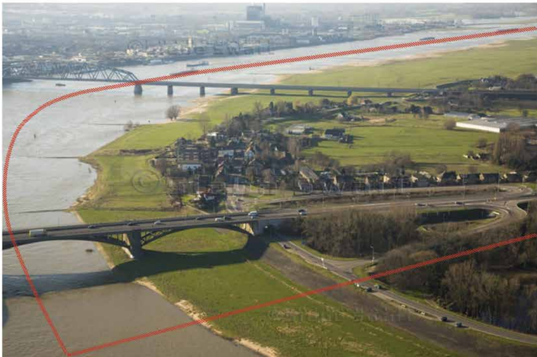
Figure 136 Discharge Capacity and Flood Frequency: Average number of days when side channel is activated and increase of the discharge capacity of the Waal river by about 1/3 when the discharge at Lobith reaches 16000 m 3 /s (10.165 m 3 /s along Waal) (based on Spatial Plan, Nijmegen, 2007) and Project Site (Photo: Siebe Swart)
