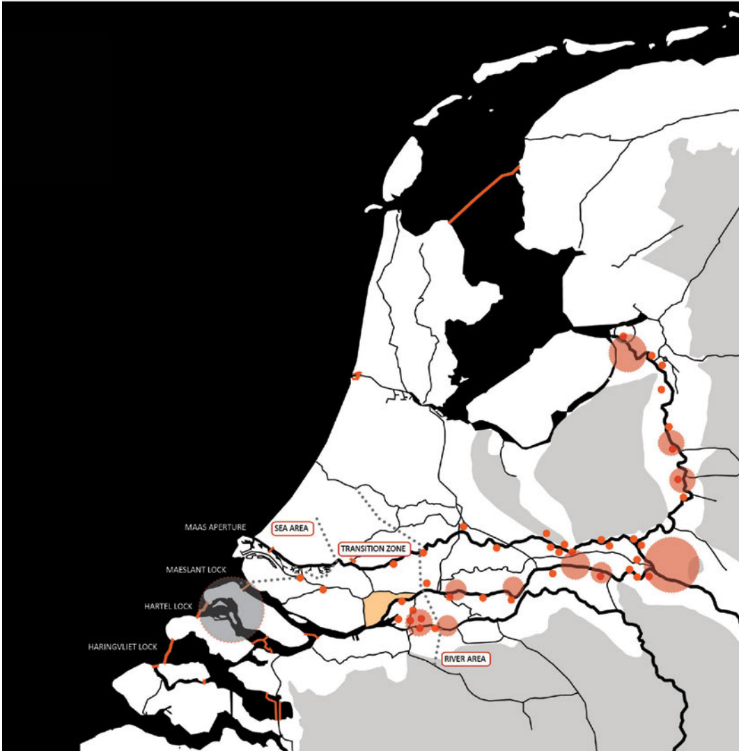
Figure 105 'Afsluitbaar Open'- Concept for the Rijnmond Island (Ties Rijcken, TU Delft, source: Deltacommissie, 2008) and Dordrecht's location in the transition zone between the sea-dominated and river-dominated delta with Room for the River measures and locks and potential sites for future RvR measures (original graphic: Bax et al, 2008, Pelt et al, 2011:11,29 adapted by author).
