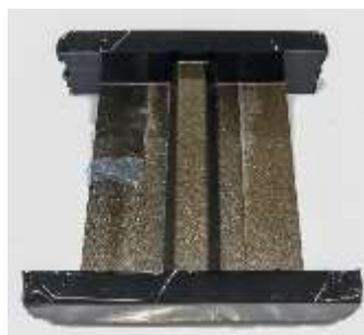
Figure 2. Single-stringer specimens before the test.
