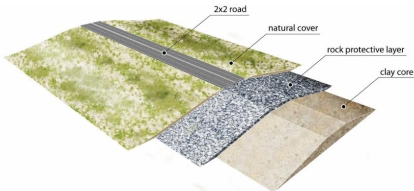
Figure 17 - Layered cross section of dike-in-dune concept for the preferred design
