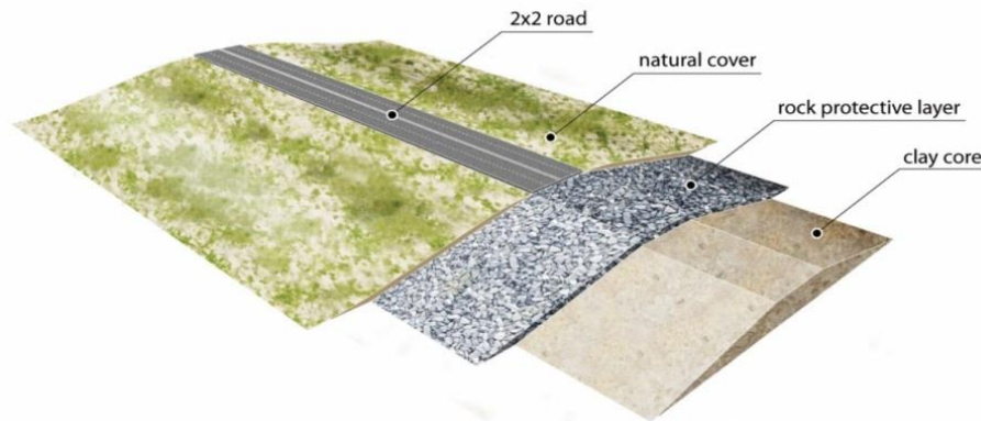
Figure 3 - main concept of the 'Dike-in-dune' land barrier design
