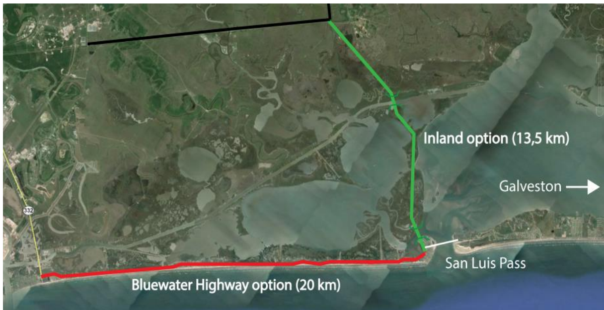
Figure 24 - Feasible alternatives for land barrier western end
