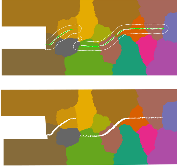
Figure 5.5: Rail shear test: the final iso-0 and skeleton curves (top), and the final deformed configuration (bottom) in the mesh partitioned into 15 subdomains.
