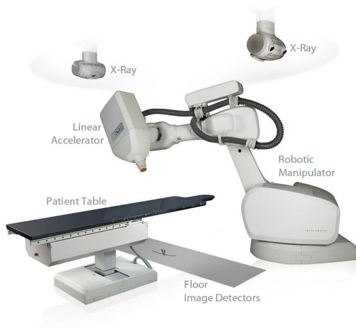
Figure 7.1: CyberKnife shown with the two X-ray detectors.
