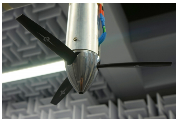
FIG. 6. (Color online) Propeller used in the experiments (3-blade Master Aircscrew E-MA1260T).
