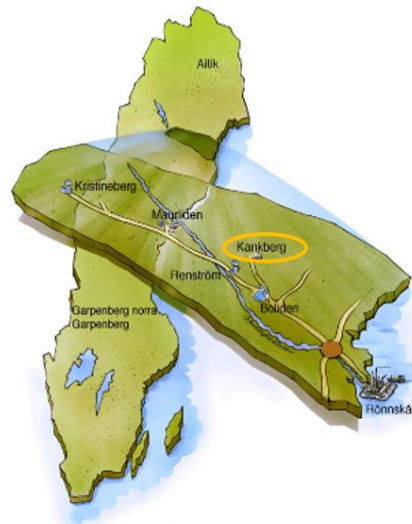
Figure 10: Boliden mining operations in Västerbotten county with three underground mines Kristineberg, Renström & Kankberg. The processing plant is located in Boliden and smelter in Rönnskär (New Boliden ).
