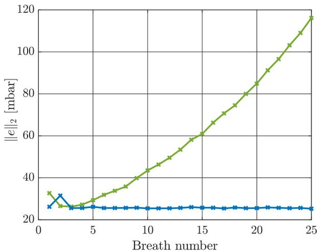
Fig. 11.  $\ell^2$ -norm of the error for every breath for  $n_o = 0$  (—), and  $n_o = 20$  (—) for the baby use case. The figure shows unstable behavior for that the closed-loop system with  $n_o = 20$ .
