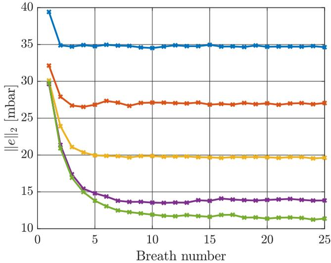
Fig. 9.  $\ell^2$ -norm of the error for every breath for  $n_o = 0$  (—),  $n_o = 1$  (—),  $n_o = 5$  (—),  $n_o = 15$  (—), and  $n_o = 20$  (—). The figure shows that more oscillators result in a smaller error, and the controllers converge in approximately ten breaths.
