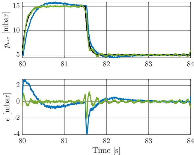
Fig. 8. Time domain results upon convergence for  $n_o = 0$  (—) and  $n_o = 20$  (—), and the target pressure (—). The figure shows that the error is significantly reduced by the repetitive controllers.
