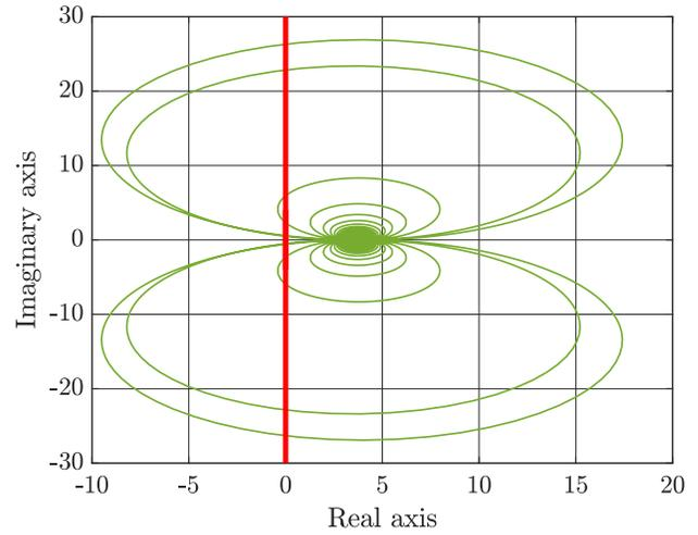
Fig. 10. Nyquist plot of  $\mathcal{H}(s)$  for  $n_o = 20$  (—) for the baby use case. The figure shows that  $\text{Re}(\mathcal{H}(j\omega)) > 0 \forall \omega \in [-\infty, \infty]$  does not hold; hence, convergence is not guaranteed.
