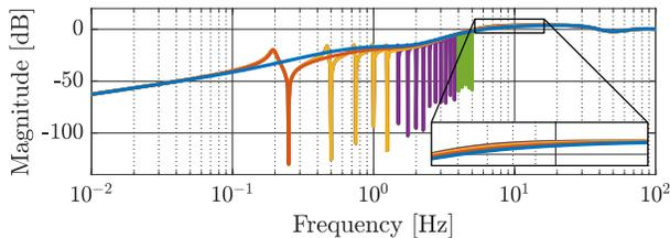
Fig. 12. Bode magnitude plot of the sensitivity  $S_{re}$  for the linearization of the closed-loop system with  $n_o = 0$  (—),  $n_o = 1$  (—),  $n_o = 5$  (—),  $n_o = 15$  (—), and  $n_o = 20$  (—). The figure shows a magnitude increase at frequencies around 8 Hz, causing oscillations at these frequencies.
