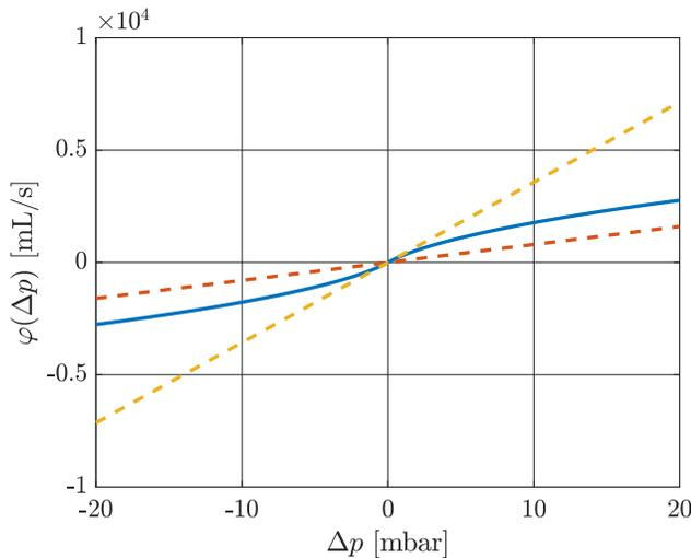
Fig. 6. Visualization of the nonlinearity  $\varphi(\Delta p)$  (—), and its sector bounds  $\underline{\varphi}\Delta p$  (---) and  $\bar{\varphi}\Delta p$  (---), showing that the incremental sector condition holds for  $[\underline{\varphi}, \bar{\varphi}] = [80, (1/R_1) + \eta]$ .
