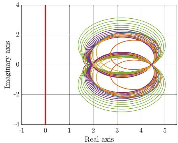
Fig. 7. Nyquist plot of  $\mathcal{H}(s)$  for  $n_o = 0$  (—),  $n_o = 1$  (—),  $n_o = 5$  (—),  $n_o = 15$  (—), and  $n_o = 20$  (—). The figure shows that  $\text{Re}(\mathcal{H}(j\omega)) > 0 \forall \omega \in [-\infty, \infty]$ .
