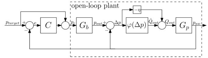
Fig. 4. Block diagram of the full ventilation system, with  $G_b$  the blower dynamics,  $C$  an arbitrary feedback controller,  $G_p$  the patient-leak dynamics, and  $\varphi(\Delta p) = R_{hose}(\Delta p) + \eta\Delta p$  the nonlinear hose model.
