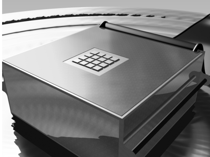
Figure 4.3: The phased array antenna mounted on the instrument box
