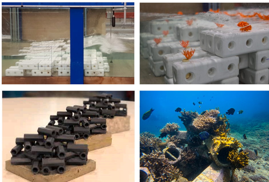
Fig. 1. Examples of artificial reef units: Upper: Reef enhancing breakwater by Reefy in wave flume (source: Van den Brekel, 2021); Lower: Moses by ReefSystems (Lower left: model tests by Van Dieren, 2022; Lower-right: application in practice).
