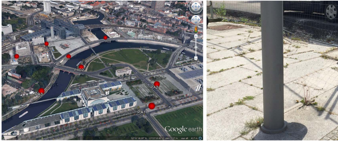
Fig. 4. (Left) Selected reference point candidates visualized as red dots in the optical image of Berlin (Google Earth). All of the candidates are assumed base of lamp posts. (Right) Photograph of one of such lamp posts in Berlin.
