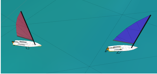
Figure 7: Mesh resolution of single mesh at highest resolution supported by Unity (65536 vertices) in which whole boats still sit on individual triangles
