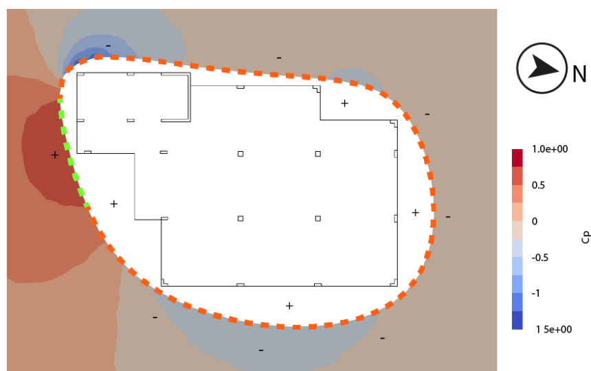
Figure 8.4: Horizontal slice at 3.7 m above ground level of Figure 8.3b showing the cp-values
