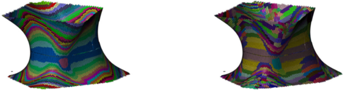
Figure 4.4: Panelisation with seven (left) and 49 families (right) [37]
