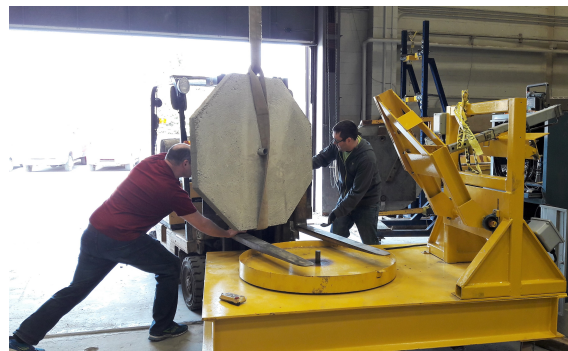
Figure 3.7: Concrete slab positioning on turntable
