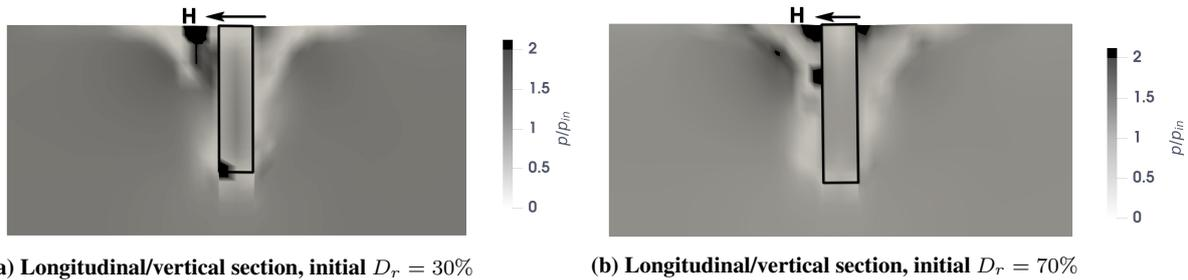
**Fig. 11.** Distribution of the  $p/p_{in}$  ratio between the final ( $N = 100$ , nil lateral load) and the initial (after gravity loading) values of mean effective stress – simulation cases (a) L2 and (b) D2.
