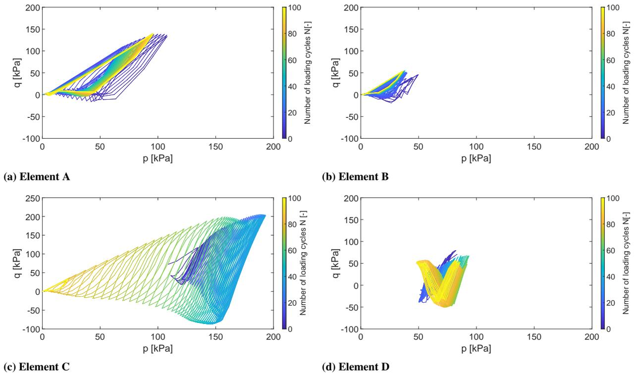
**Fig. 10.** Cyclic effective stress paths at the reference elements in Fig. 2. Values of mean and deviatoric stress invariants were obtained from the effective stress tensor ( $\sigma_{ij}$ ) and deviatoric ( $s_{ij}$ ) effective stress tensors as  $\sigma_{kk}/3$  and  $\sqrt{(3/2)s_{ij}s_{ij}} \cdot \cos(3\theta_\sigma)$ , respectively, where  $\theta_\sigma$  stands for the Lode angle. Simulation case D2.
