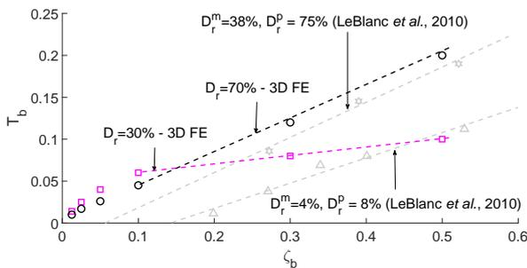
**Fig. 14.** Comparison between experimental (1g) and numerical  $T_b - \zeta_b$  trends for loose and dense sand – pure one one-way cyclic loading ( $\zeta_c = 0$ ). Relative density values for the reference test data are provided for model ( $D_r^m$ ) and prototype ( $D_r^p$ ) scales as per **LeBlanc *et al.* (2010)**.
