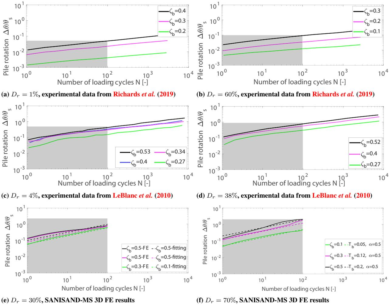
**Fig. 12.** Influence of the cyclic load amplitude ratio ( $\zeta_b$ ) on the normalised pile rotation ( $\Delta\theta/\theta_s$ ) against the number of loading cycles ( $N$ ). Both Experimental and 3D FE results correspond with pure one-way cyclic loading ( $\zeta_c = 0$ ).
