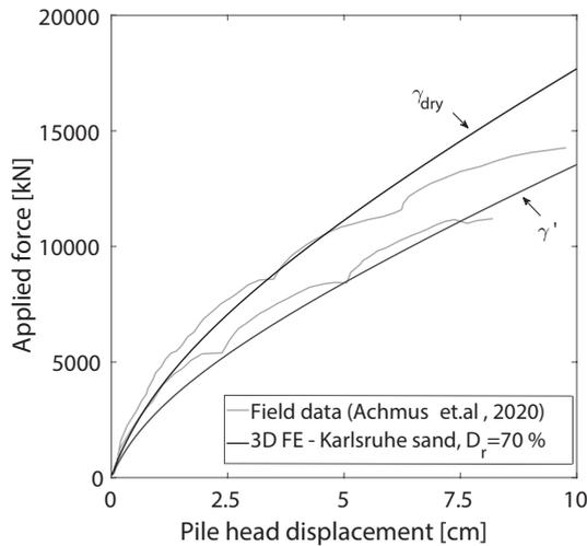
**Fig. 3. Comparison between monotonic monopile responses from 3D FE modelling (Karlsruhe sand,  $D_r = 70\%$  -  $\gamma_{dry} = 15.3 \text{ kN/m}^3$  and  $\gamma' = 9.4 \text{ kN/m}^3$ ) and field testing (from Achmus *et al.* (2020), piles P3-P4).**
