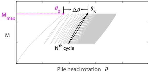
Fig. 6. Definition of reference pile rotation values.
