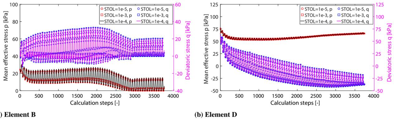
**Fig. 18. Influence of  $STOL$  (tolerance for error-driven sub-stepping) on stress integration at elements B and D in Fig. 2 – simulation case L2 in Table 3. Values of mean and deviatoric stress invariants were obtained from the total ( $\sigma_{ij}$ ) and deviatoric ( $s_{ij}$ ) effective stress tensors as  $\sigma_{kk}/3$  and  $\sqrt{(3/2)s_{ij}s_{ij}} \cdot \cos(3\theta_\sigma)$ , respectively, where  $\theta_\sigma$  stands for the Lode angle.**
