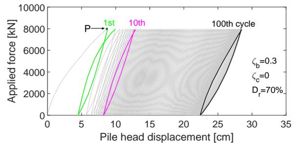
(a) Lateral force vs pile head displacement ( $D_r = 70\%$ )
