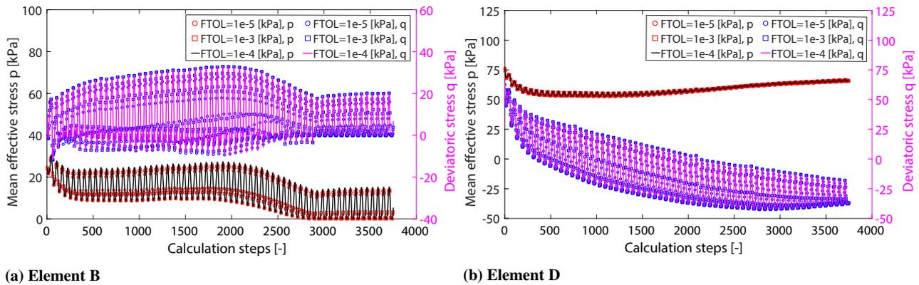
**Fig. 19. Influence of  $FTOL$  (tolerance for the yielding test) on stress integration at elements B and D in Fig. 2 – simulation case L2 in Table 3. Values of mean and deviatoric stress invariants were obtained from the total ( $\sigma_{ij}$ ) and deviatoric ( $s_{ij}$ ) effective stress tensors as  $\sigma_{kk}/3$  and  $\sqrt{(3/2)s_{ij}s_{ij}} \cdot \cos(3\theta_\sigma)$ , respectively, where  $\theta_\sigma$  stands for the Lode angle.**
