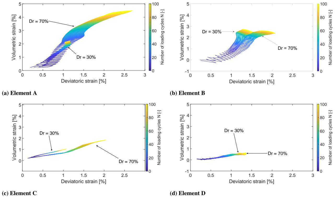
**Fig. 8.** Cyclic strain paths at the reference elements in Fig. 2. Values of volumetric and deviatoric strain invariants were obtained from the total ( $\varepsilon_{ij}$ ) and deviatoric ( $e_{ij}$ ) strain tensors as  $\varepsilon_{kk}$  and  $\sqrt{(2/3)e_{ij}e_{ij}}$ , respectively. Simulation cases L2 and D2.
