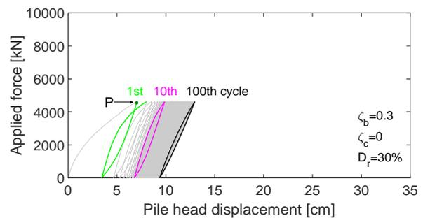
(b) Lateral force vs pile head displacement ( $D_r = 30\%$ )
