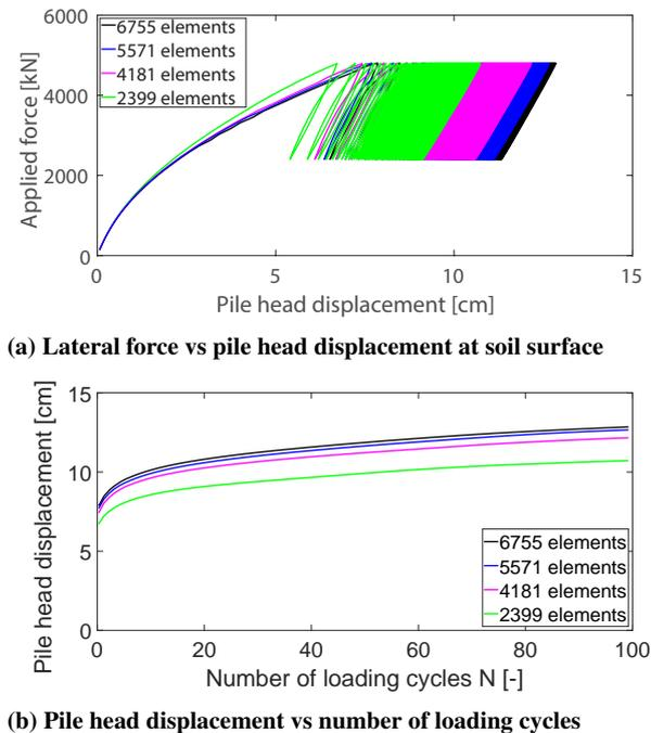
**Fig. 17. Mesh sensitivity effects in the monopile response to lateral cyclic loading ( $D_r = 30\%$ , simulation case L6 in Table 3).**
