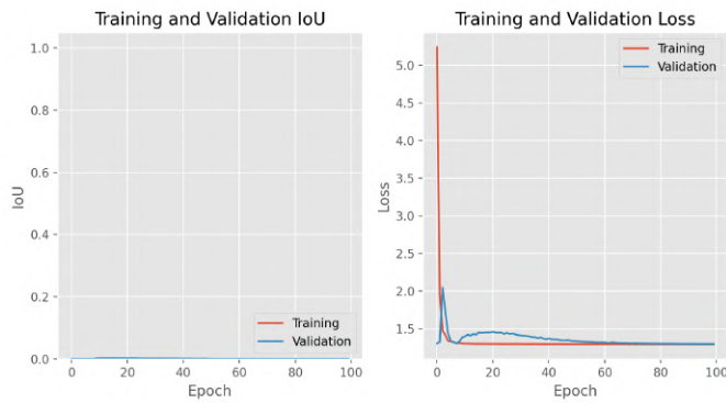
Figure 4.12: Learning curve showing the loss and the Mean Intersection over Union (mIoU) for the A_{ratio} representation from the U-Net. The batch size for this test was 64.
