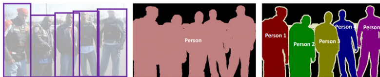
Figure 2.5: left to right; object detection, semantic segmentation, instance segmentation. Source: [Gkioxari et al.].
