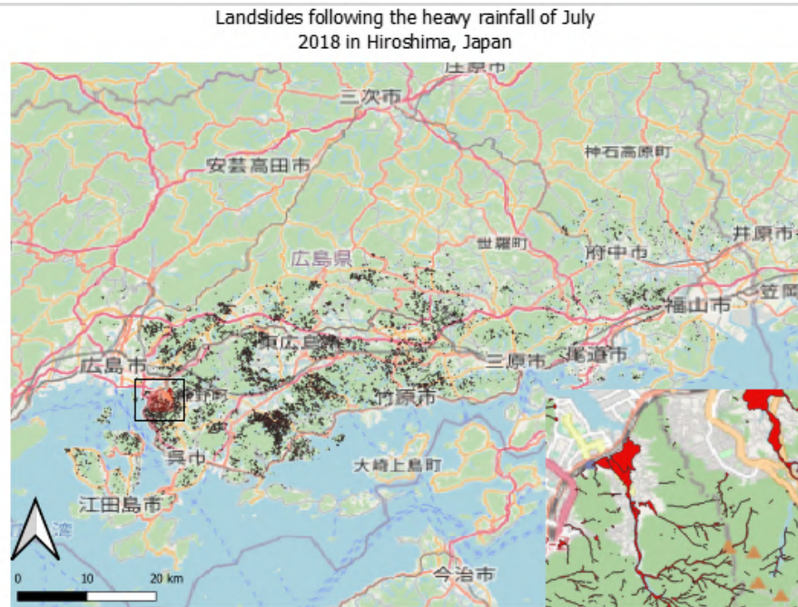
Figure 3.4: The landslide database in Hiroshima, Japan. The red polygons (in the zoomed in figure these appear red, in the larger figure these are more black) are landslides.
