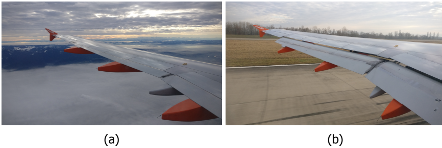
Figure 1.4: Wing of an Airbus A320 aircraft showing the flap fairings [20]. a) Flaps retracted during cruise; b) Flaps extended during landing.
