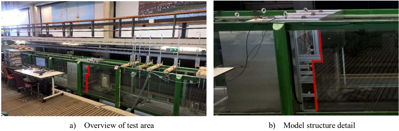
Fig. 6. Experimental test area. a) Overview of the wave flume, impact structure (highlighted in red), instrumentation and acquisition systems. b) Detail of aluminium impact surface (highlighted in red) and concrete support block.
