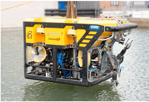
Fig. 12. iTech 7 Centurion SP ROV being deployed for a mission [115–117].
