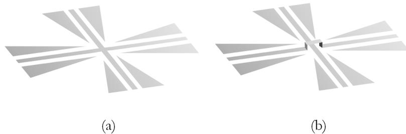
Figure 7.32: Proposed CPW fed dual polarized leaky slot geometries: (a) The ordinary design and (b) the modified design with airgap located at the center, separating the crossing CPW lines.
