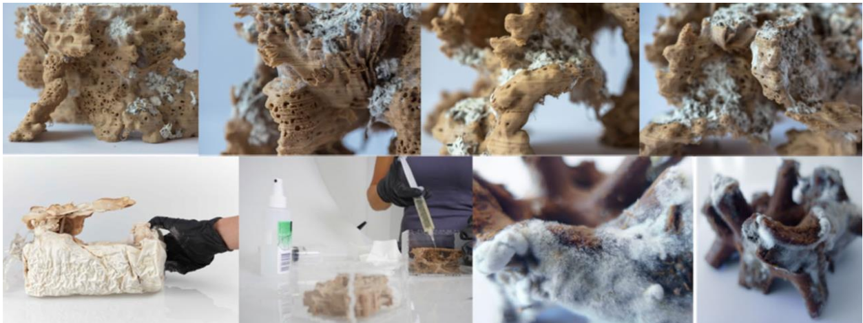
fig. 09. “Bio Scaffolds” – prototypes of 3d printed wood structures infused by mycellium, RMIT, Natalie Alima
