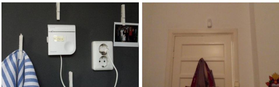
Fig. 1. T, CO 2 , RH box (left) and movement sensor (right) as used during the Ecommon measurement campaign.
