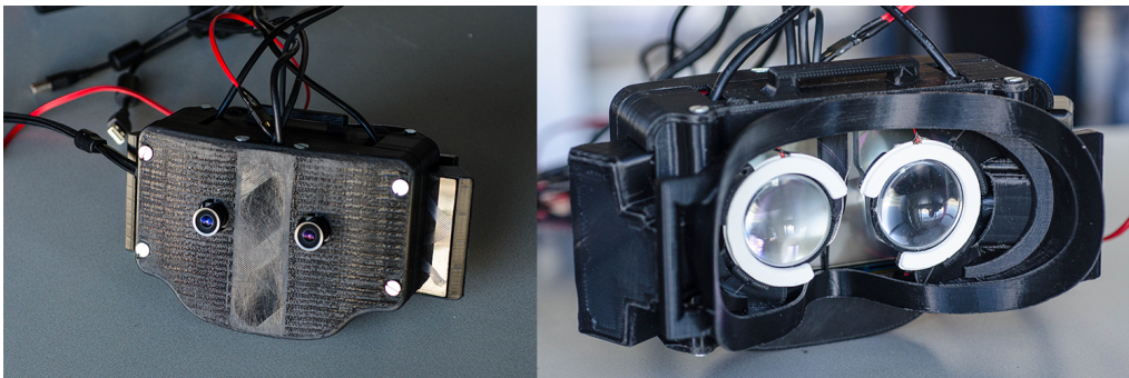
Figure 1.1: A custom designed and 3D printed HMD, viewed from the front (left) and from the back (right)
