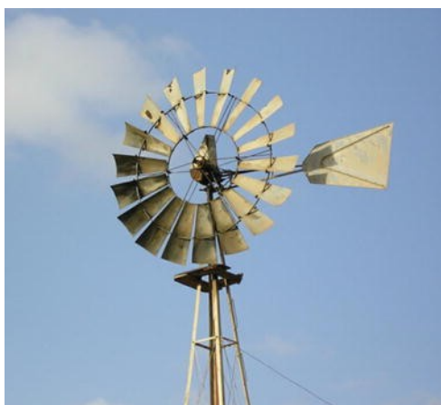
Figure 2.4: A typical American windmill to pump water [36].
