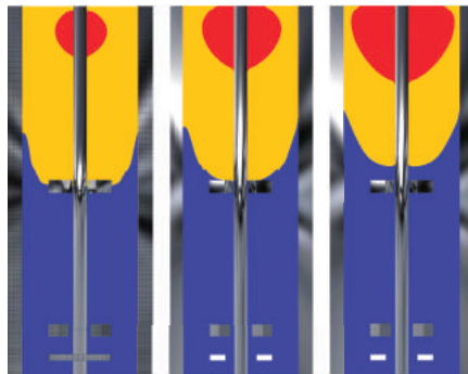
Figure C1: Variation of the regime layout as a function of the circulation time. Left: regular settings ( \tau_{circ} = 18.2 s). Middle: case SENS – 1 ( \tau_{circ} = 25.6 s). Right: case SENS – 2 ( \tau_{circ} = 18.2 s).
