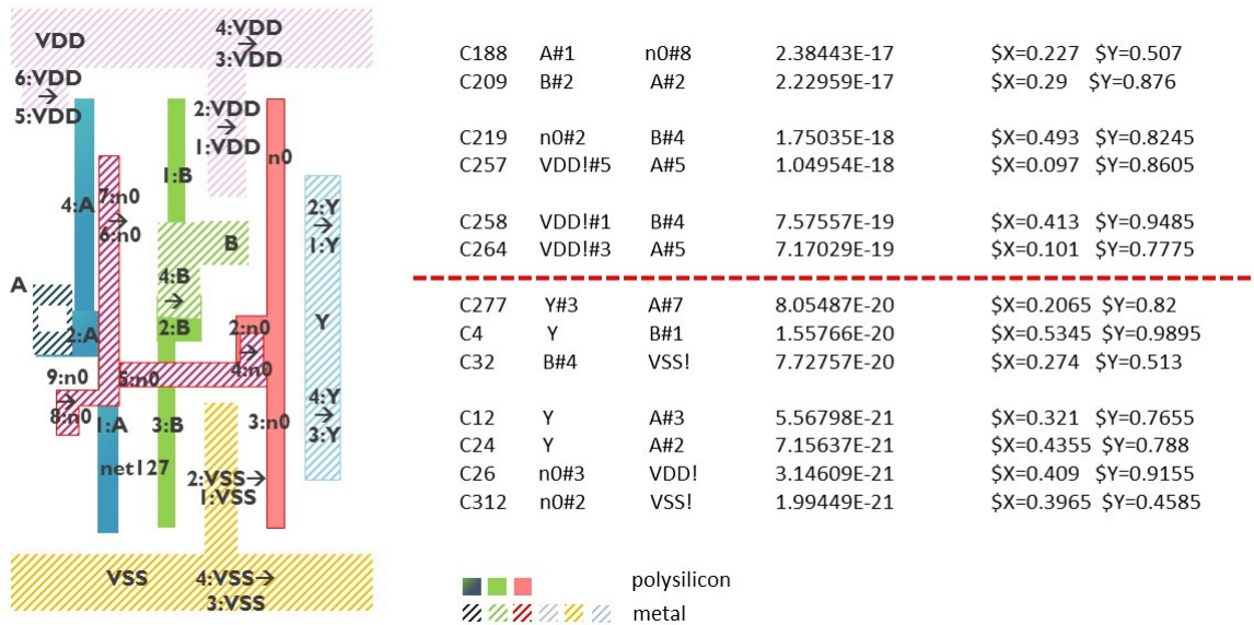
Figure 5.3: AND2X1 layout to illustrate heuristics for choosing C_{th}
