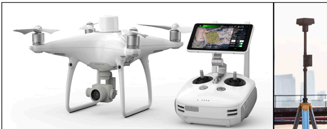
Figure 4. DJI Phantom 4 RTK: drone and remote controller (left); DJI RTK base-station (right) [91].
