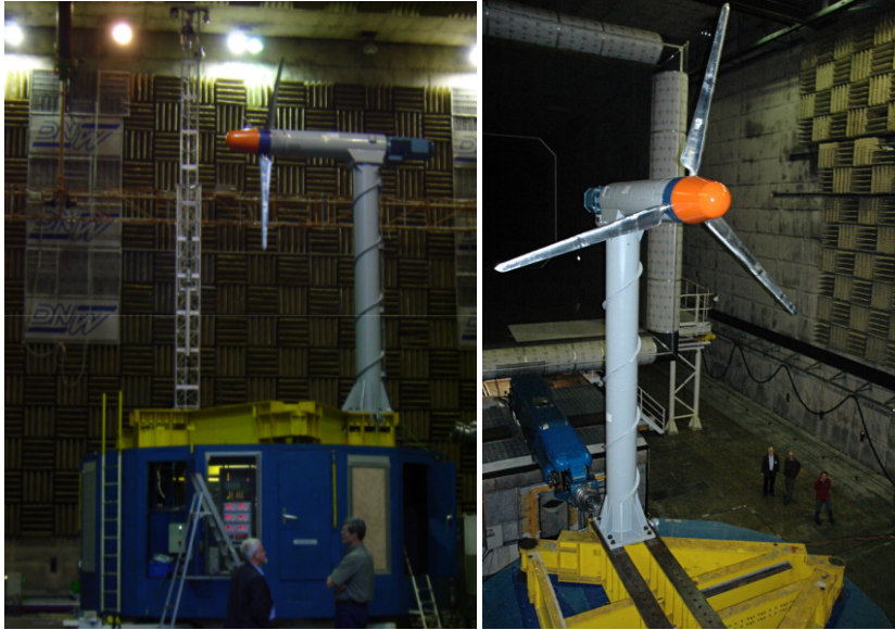
Figure 1.7: The MEXICO Wind turbine test set-up in the DNW wind tunnel (Scheepers and Snel, 2007)
