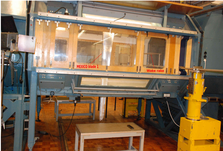
Figure 4.6: Experimental set-up of the model: the MEXICO blade 1
