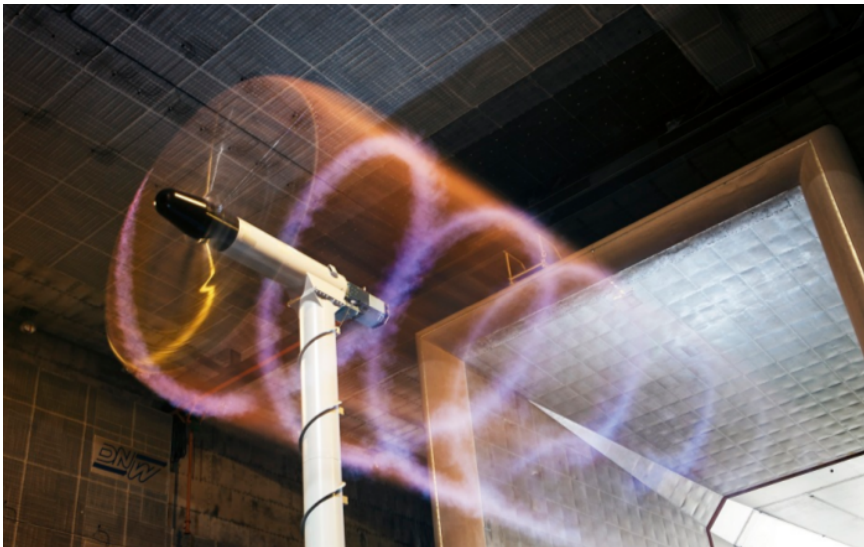
Figure 1.1: Smoke visualization of tip vortices generated from the blade tip in the second phase of MEXICO experiment (Boorsma and Schepers, 2014)
