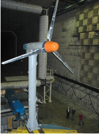
Figure 5.1: The MEXICO experiment in DNW wind tunnel (Snel et al., 2007). Three bladed wind turbine with 4.5m diameter rotor.
