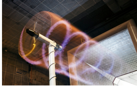
Figure 5.2: Smoke visualization of tip vortices generated from the blade tip in the second phase of MEXICO experiment (Boorsma and Schepers, 2014)
