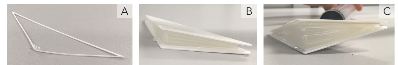
Figure 65: Iteration 4: Prototyping process - A: Rigid reinforcement structure B: Prototype with integrated reinforcement structure C: Prototype after inflation, resulting in rotation without balloon-blowing effect
