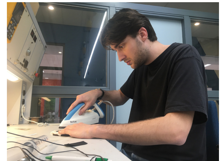
Figure 58: Heat sealing with flat iron
