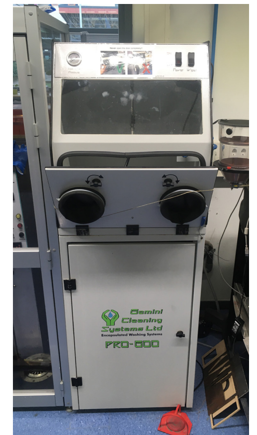
Figure 60: Waterjet for removing support material
