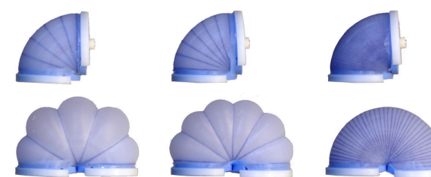
Figure 41: Silicone actuators with reinforcement fibers, showing the effect of the density of the fibers on the ballooning effect (Fras et al., 2017)
