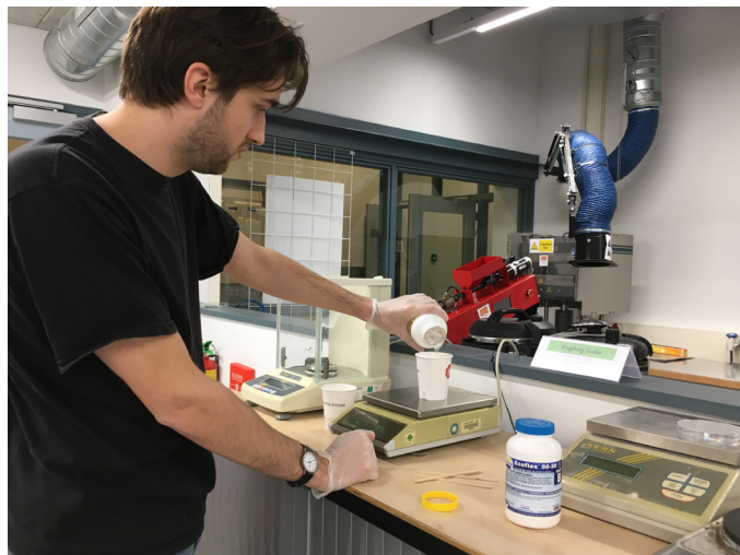
Figure 53: Weighing silicone to obtain 1:1 ratio
