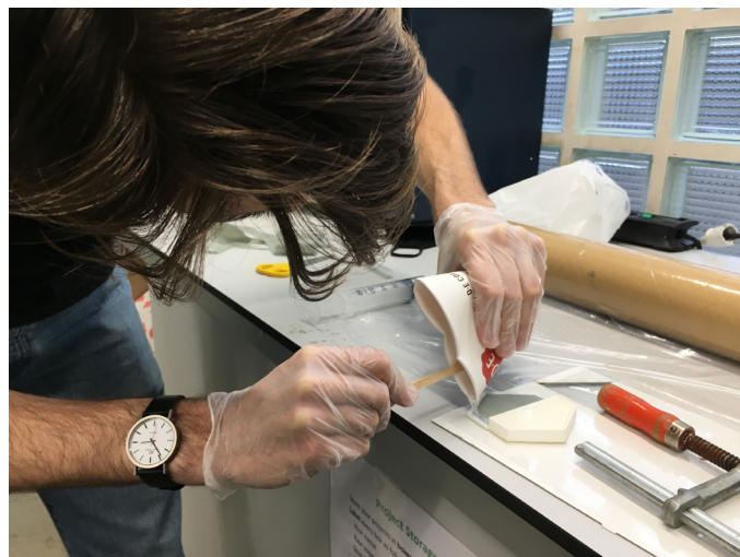
Figure 55: Casting silicone into a mold
