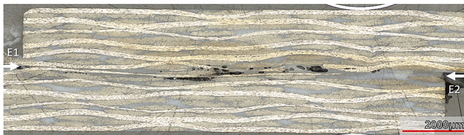
Fig. 12. Longitudinal cross-section micrographs of the highest strength weld for case DED-HF(A) with consolidation force of 1500 N applied for 60 s.
