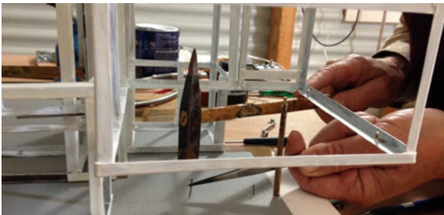
FIG. 26 The fixation with nails and the pillar turned out of brass at the corner of the ‘salle commune’ that hold the glass sides of the ‘salle commune’, on 19 May 2017. Photo Marijke Smit
