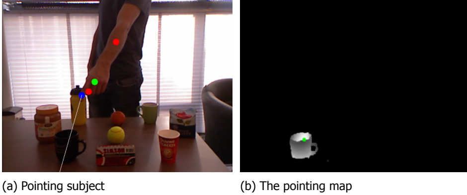
Figure 3.3: The subject is pointing at the blue coffee cup. At the left hand side the pointing direction is visualized by the line. The blue dot represent the location of the pointing finger. Furthermore the two red dots indicate the location of the elbow and the hand. The green dot in the left image shows the centroid of the hand point cloud, whereas the green dot in the right image shows the most salient point in the pointing map.
