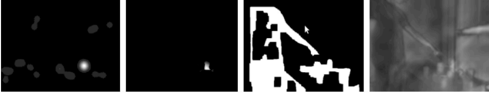
Figure 3.5: In this figure the four saliency maps are showed. From left to right the images represent the Gaze map (G), Pointing map (P), Depth map (D) and bottom-up Saliency map (S).
