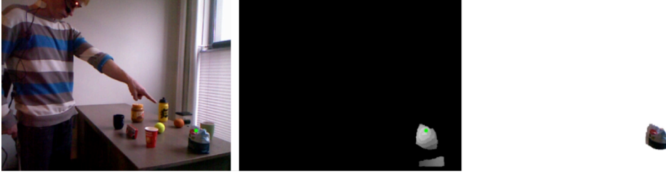
Figure 3.14: From left to right: the view from the robot, the combined saliency map and the found object of interest. The green dot indicates the most salient point in the saliency map.
