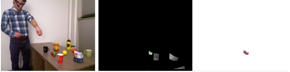
Figure 3.1: From left to right: the view from the robot, combined saliency map and the found object of interest.
