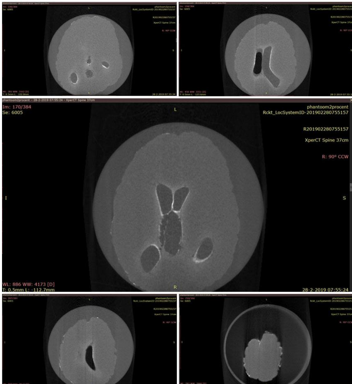
FIGURE 36 - PHANTOM WITH 2% BARIUM SULPHATE VISUALIZED USING RADIANT SHOWING DIFFERENT SLICES
