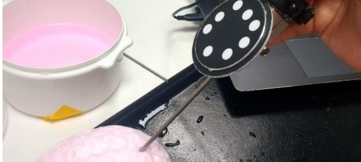
FIGURE 44 - ENDOSCOPIC INTERVENTION ON BRAIN PHANTOM
