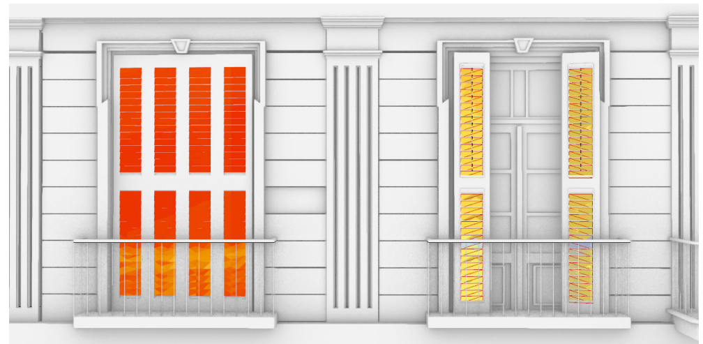
Figure (109) : Solar radiation analysis (Grasshopper&Ladybug)_Shutters
