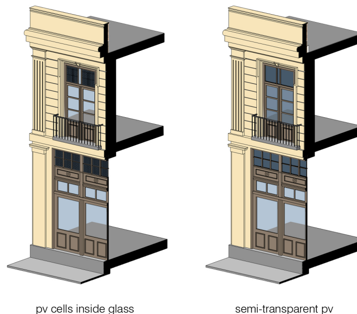
Figure (84) : Matrix window glazing options.
