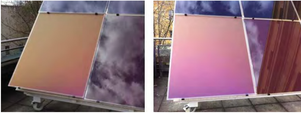
Figures (25) : Orange glass panels laminated on real-size PV modules on which strong angular dependency of the color is observed.
