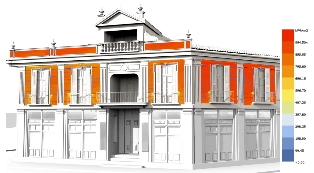
Figure (104) : Solar radiation analysis (Grasshopper&Ladybug)_Fragmented surfaces
