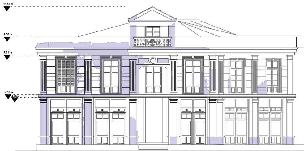
Figure (69) : Damage registration on the south-west and south-east facade (survey product)
