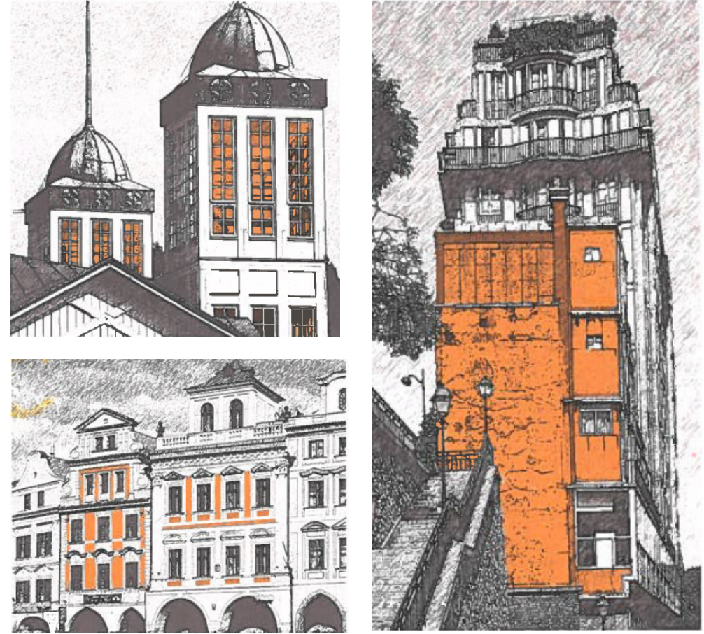
Figure (22): Examples of adequate placement of photovoltaic panels on facades. (Hermannsdörfer & Rüb, 2005).
