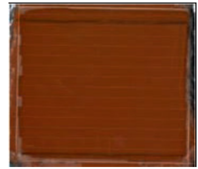
Figure (27) : Visual appearance of the amorphous module after exposure to PID. Left: condition without protecting tape after 300 h. Right: condition with protective tape after 500 h.
