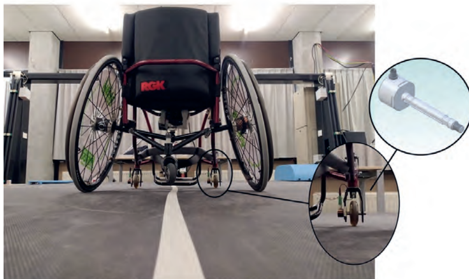
Figure 5.1a-b. Measurement set-up during the treadmill sessions. The custom-made load pins were integrated in each of the castor wheels (normal castor wheel axle were replaced by the load pins)
