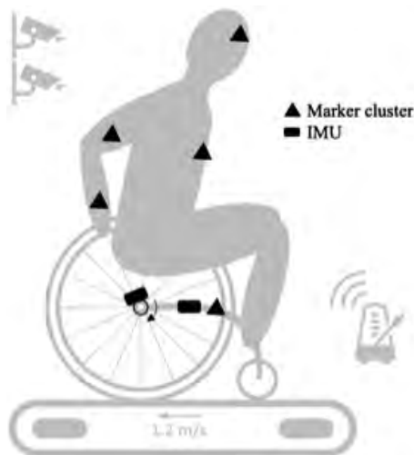
Fig. 3.2. Overview of the measurement setup. Participants were measured with a MOCAP system with marker clusters ( \Delta ) on the wheelchair frame, trunk (sternum), head, upper arm and lower arm, and IMUs ( \square ) on the wheel axle and on the center of the wheelchair frame. Both the 3.0 x 5.0m treadmill and the 1.0 x 1.0 force plate (below the treadmill) are visible in the figure.
