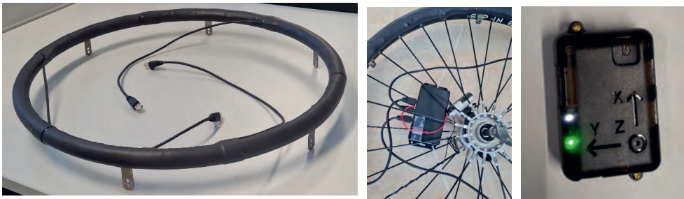
Figure 9.1a-c. The RHIDE system [prototype version November 2022] and its different components. Fig. 9.1a (left) shows the capacitive sleeve attached to a wheelchair push-rim, Fig. 9.1b (middle) shows how the cables from the capacitive sleeve connect with the left side of the microcontroller unit (black square) and the cable of the IMU (around the wheel axis) is connected via a red wire to the microcontroller unit. Fig. 9.1c (right) shows the IMU.
